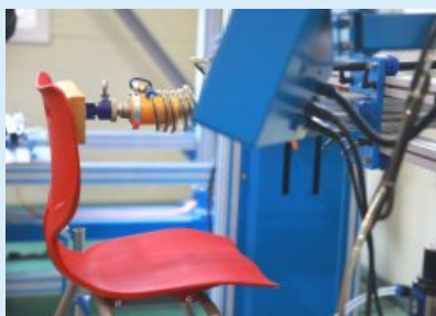
An In-house quality testing room (* Equipment: a backrest strength tester, a drop impact tester, a repeated impact tester, and a repeated opening and closing tester)
